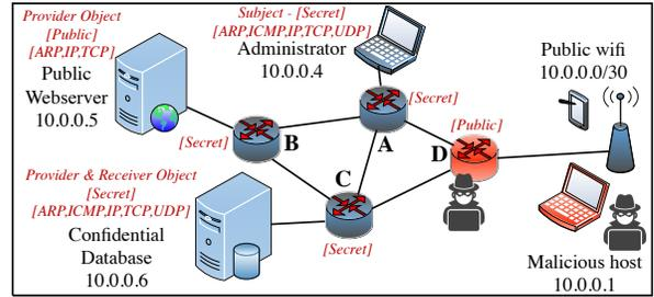
Fig. 5. Experimental network setup with assigned security labels. Using the SDNMap scanner, the (Public) adversary was only able to identify the other Public node in the network, where *MLSNet* prevented any higher-level traffic from ever reaching them, thus limiting their ability to reconstruct flow rules.
